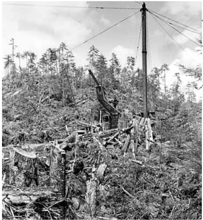
Taken in 1968, this photo shows a slightly more modern steel spar and a heel boom loader.
